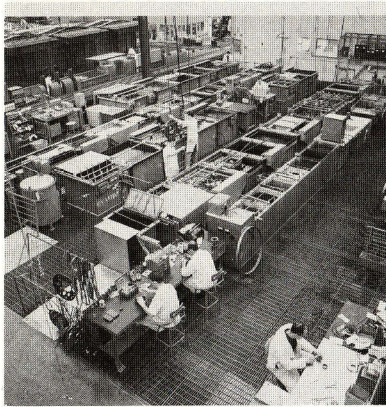
The Heat Treat and Process Shop performs copper, cadmium, chrome, nickel, silver and lead-plating of engine parts and components.
